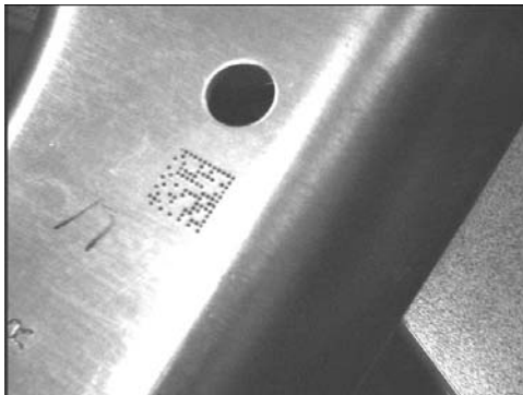
Individual Part Marked with Data Matrix
